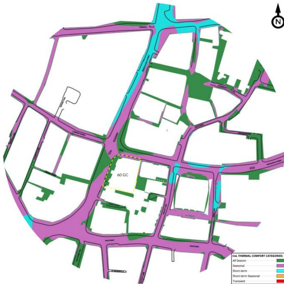
Figure 8. Existing Baseline - Ground Level, Annual Thermal Comfort Conditions
